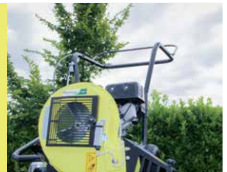
AS440 - composed of side exit nozzle and protection grid (not usable in models with side brush)
