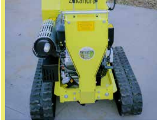
Great stability thanks to quality tracks produced in Italy , 1050 mm length; 900 mm track.
