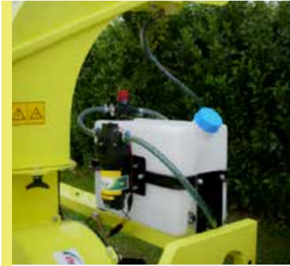
COD. OL1300 Humidifier kit for dust suppressions
