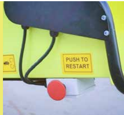
Emergency/ re-start buttons.
