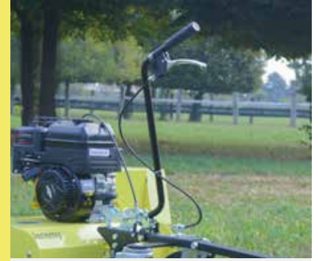
Automatically operated lifting handle for the cutting system.
