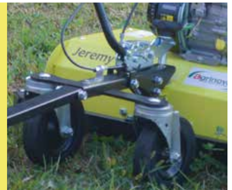
2 front pivoting solid rubber wheels with sheet metal rims.
