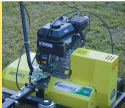
Central engine position for optimum weight balance.
