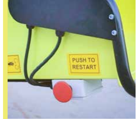
Emergency/ re-start buttons.
