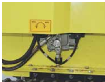
Possibility of adjusting the feed roller speed by acting on the flow adjustment knob.
