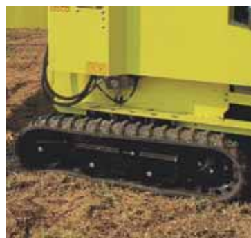
Great stability thanks to quality tracks produced in Italy. - 1 mt track.
