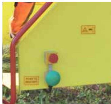
Emergency/ re-start buttons.
