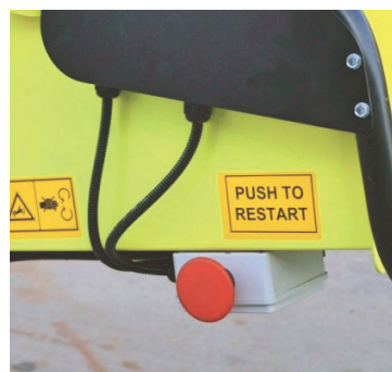
Emergency/ re-start buttons.
