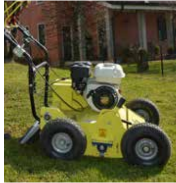
Tires: 4 tires 280 mm diametre, 100 mm wide
