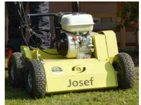
Good stability thanks central position of engine
