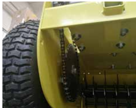
Differential system: obtained with freewheel sprocket and chain drive
