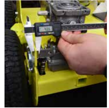
Chassis 4 mm thickness
