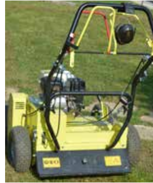
Adjusting levers: 7 far blades engaging 7 far self propelling 1 far speed regulation (updating)
