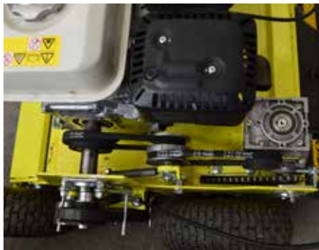
Speed regulation: the variation of speed is obtained through axial shifting of central pulley driven by a self-lubricating bush. Variable speed from 0 up to 4,5 km/h.
