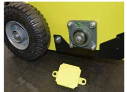
The cutting system is supported by two cast iron supports and two high quality ball bearings. The greaser, during maintenance, is easy to reach.
