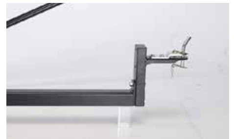
Adjustable helm attachment to facilitate coupling with any type of tractor or quad.
