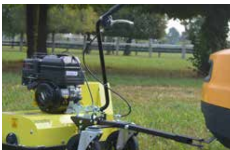
Lifting handel and automatic starting of cutting system.
