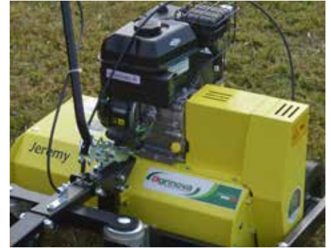
The central position of the engine, allows an excellent weigh balance
